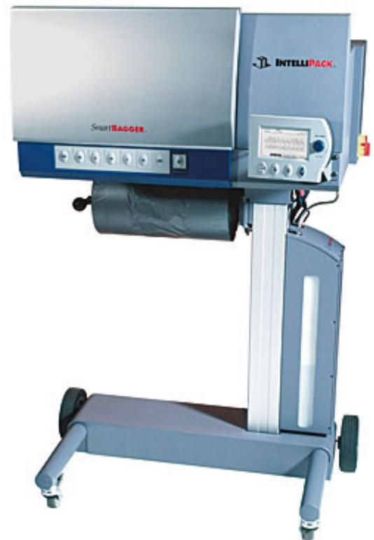
The telemetry capability on a Foam-In-Place system is similar. The unit automatically collects, monitors and measures critical information, such as liquid foam and film usage, temperature, pressure and other system parameters, each time it is operated.
